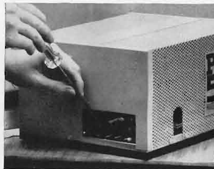
It's a tight squeeze to get at the phono input connector and loudspeaker terminals on the Peri-50 amplifier.
